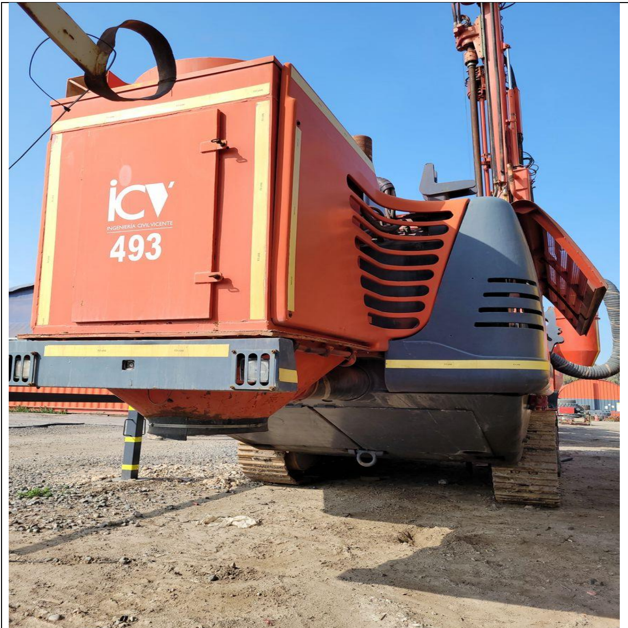
The equipment does not show damage due to impact, structure in general in good condition
