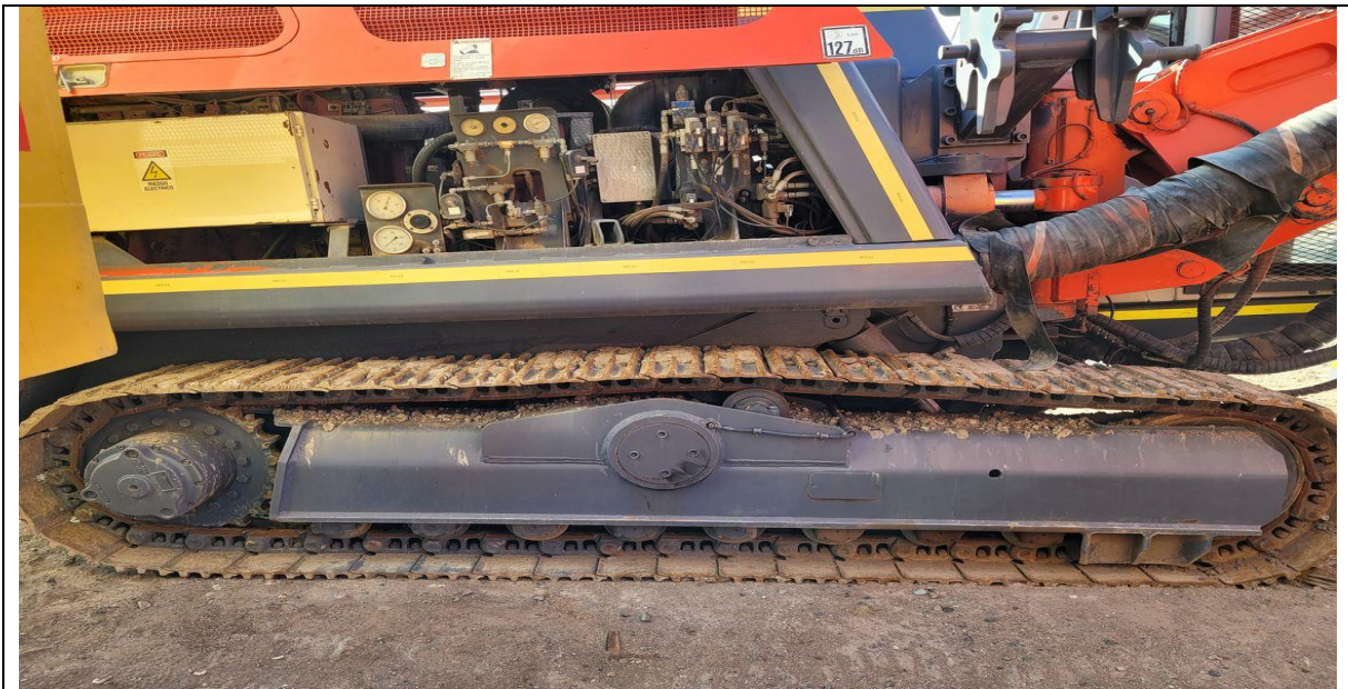
Frames in general are in good condition, they do not show cracks or abnormal wear.
