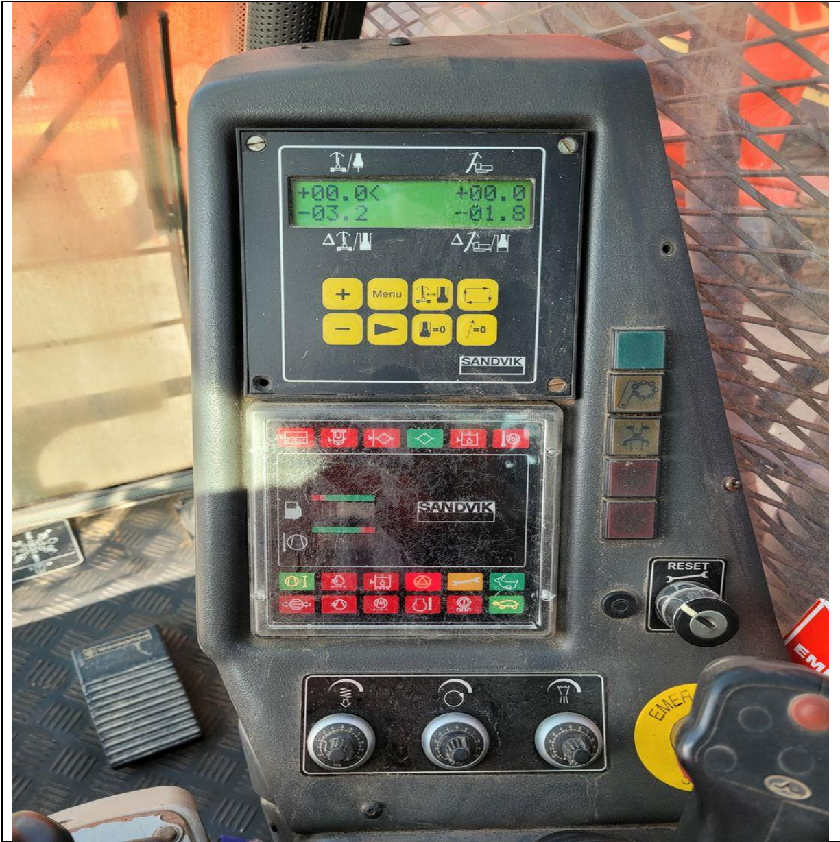
Control panel does not maintain active alarms, inclinometer working normally
