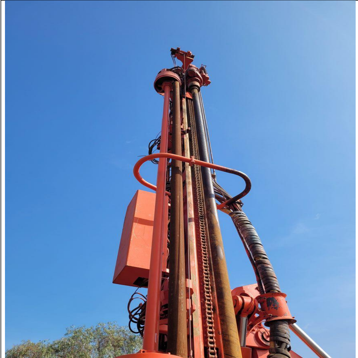
Rod handler in good condition, feed chain shows some rust
