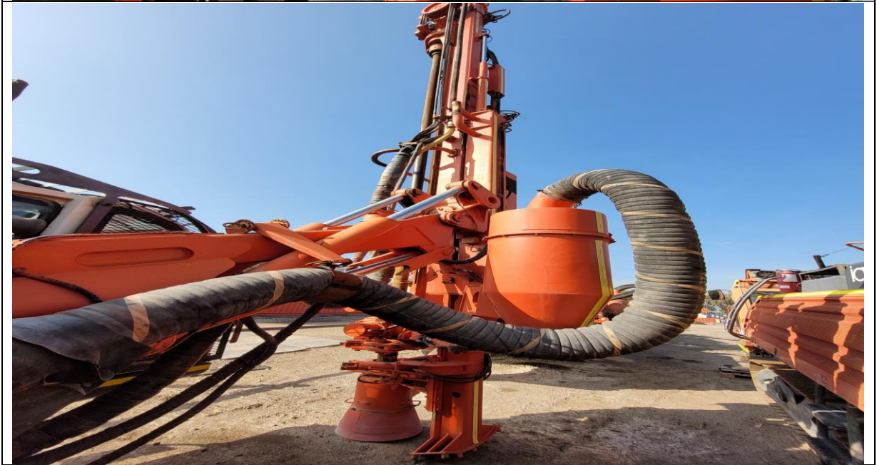
Hydraulic cylinders do not show oil leaks, chrome rods in good condition
