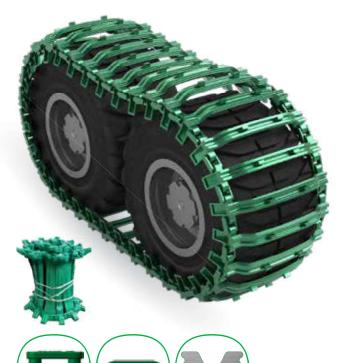
Special form of a profile, which enables an excellent traction and stability of the machine on various types of the foundation. It is appropriate for steep and stony terrains and also for mud and snow.
