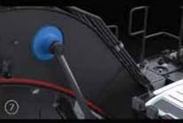
Reinforced boom cylinder cast bearing
