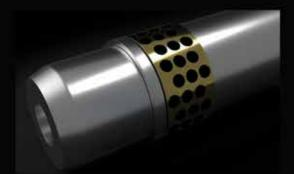
Bronze-graphite bushings used in boomarm and boom-frame connection points increase the lubrication period, and greatly prevent the wear of the pins because of graphite, having a very high grease absorption and retention capability, embedded in the inner structure of the bushings.
