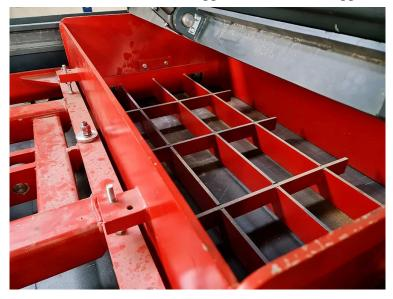
Door hopper opening by hydraulic cylinder (electrical motor option) that is filling the filling box with concrete. Opening of the hopper door to fill concrete in filler box is controlled by PLC and opening time can be programmed in the terms of quantity and time of hold. Main mix frame of base concrete is de-attachable for fast and simple maintenance of the central part of the machine.
