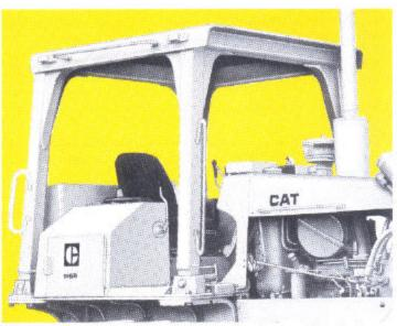
The cab contains many standard operator comfort features: air pressurizer and filter, windshield washers and wipers, tinted glass, dome light and floor mat. Air conditioner and heater are available as options. A cab accessory group is also available including coat hook, sun visor and ash tray.
